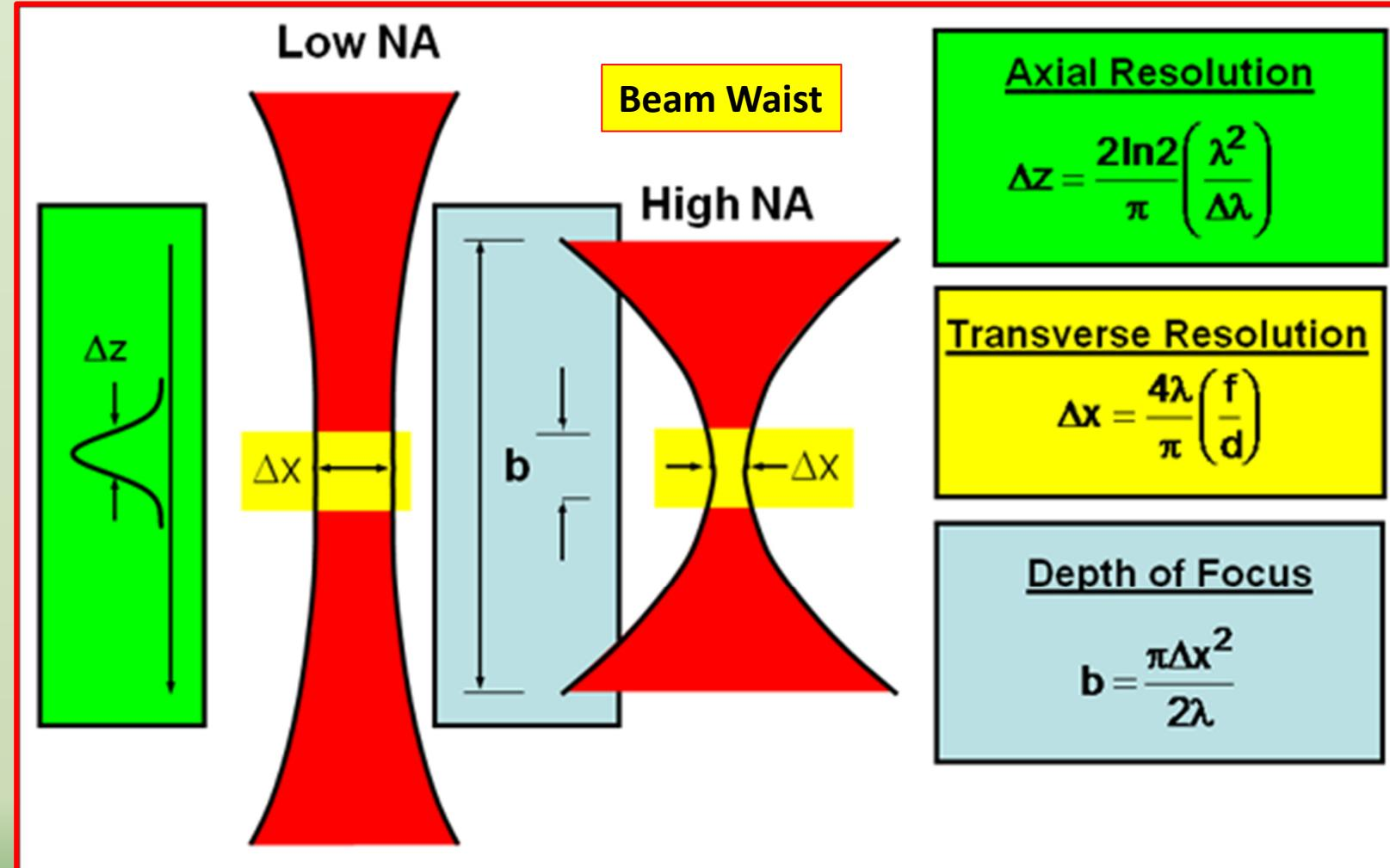
OCT can achieve high axial resolutions independent of numerical aperture. Using low coherence interferometry, the axial resolution is inversely proportional to the bandwidth of the light source. The transverse resolution is given by the focus spot size. The depth of field is determined by the confocal parameter of the focused beam
