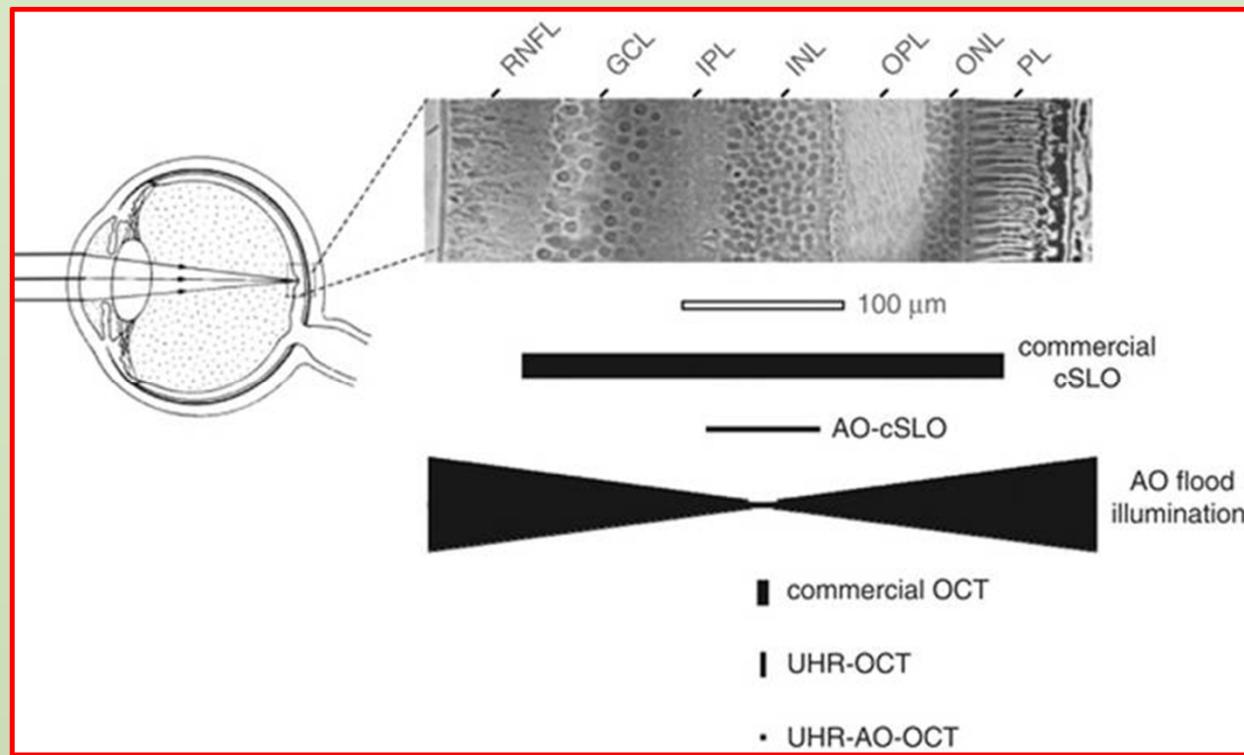
Examples shown include the commercial confocal scanning laser ophthalmoscope (**cSLO**), confocal scanning laser ophthalmoscope with adaptive optics (**AO-cSLO**), flood illumination with adaptive optics, commercial OCT, ultrahigh-resolution **OCT** (**UHR-OCT**), and ultrahigh-resolution OCT with adaptive optics (**UHR-AO-OCT**).
