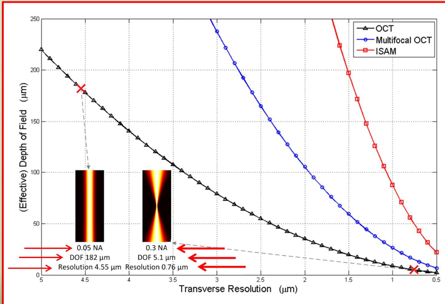
**Trade-off** between the effective DOF, Depth Of Field, and Transverse Resolution in OCT Multifocal OCT and ISAM, Interferometric Synthetic Aperture Microscopy, at wavelength of 1 μm and whth refractive index of 1.4
